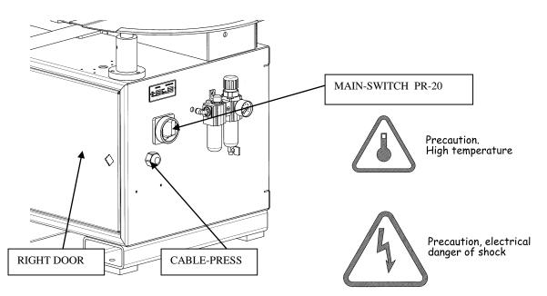
To make the connection, insert the cables from the main supply in the terminals L1 and L2 (MAIN SWITCH), securing them with the cable-press and fixing the earth cable using the appropriate nut. Connection is via terminals, and the cable cross-section must be at least 2.5mm.
